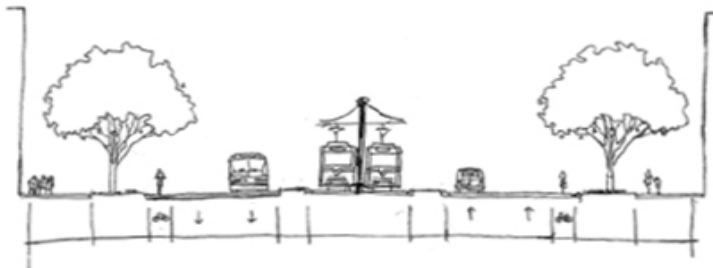
A cross-section of the future North Temple shows a 10 foot wide sidewalk, an 8 foot wide park strip, a bike lane, two vehicle lanes, and the light rail down the middle of the street.
